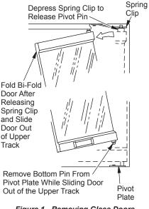
Figure 1 - Removing Glass Doors
